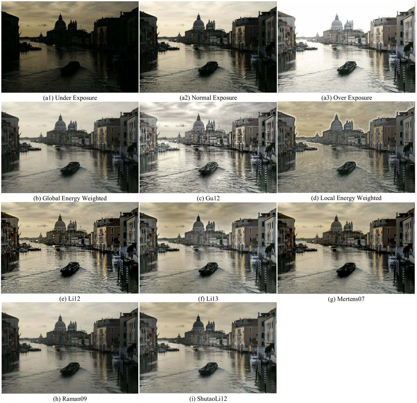
Fig. 2. An example of multi-exposure source image sequence (a1, a2, a3) and fused images (b)-(i) created by different MEF algorithms.
