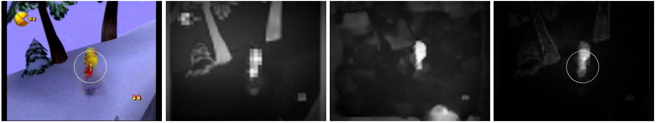
Fig. 4. Sample saliency maps. Column 1: original video frame with human fixation point marked with a circle; Column 2 - 4: spatial, temporal, and overall saliency maps, respectively.
