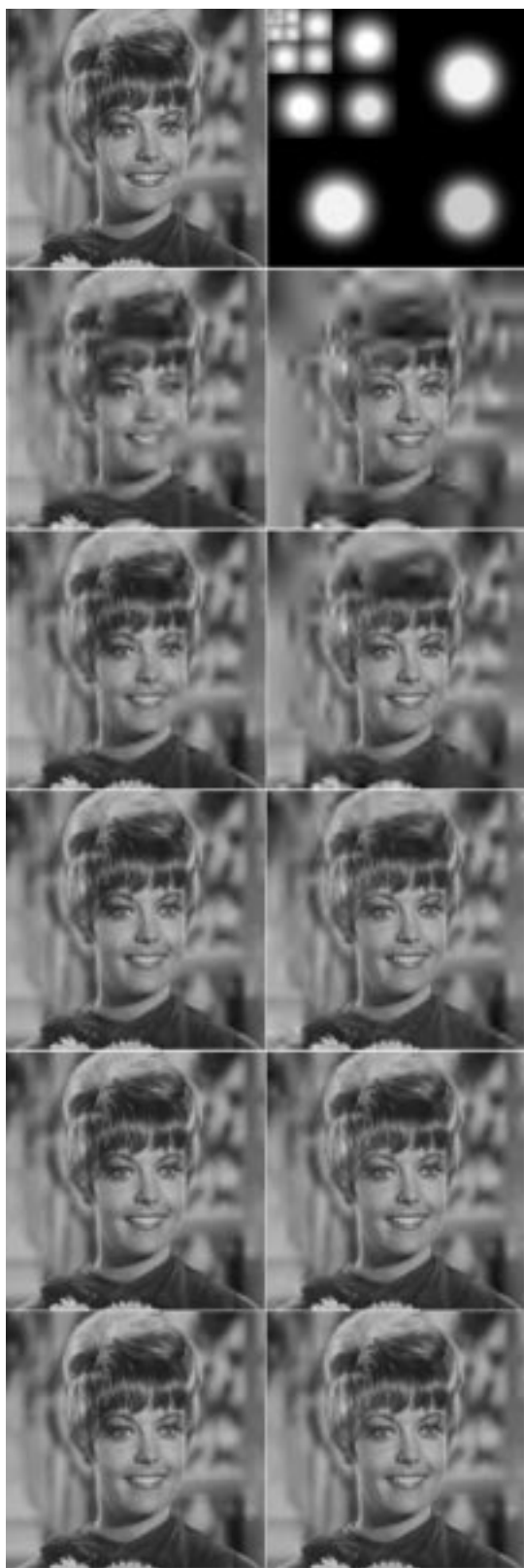
Fig. 13. "Zelda" image compression results. Top-left: original image with the foveation region indicated. Top-right: DWT domain importance weighting mask for EFIC (brightness logarithmically enhanced for display purpose). The images of the left column that follow: SPIHT coded images. The images of the right column that follow: EFIC coded images. The bit-rates from top to bottom are 0.015 625 b/p (CR = 512 : 1), 0.031 25 b/p (CR = 256 : 1), 0.0625 b/p (CR = 128 : 1), 0.125 b/p (CR = 64 : 1), and 0.25 b/p (CR = 32 : 1), respectively.
