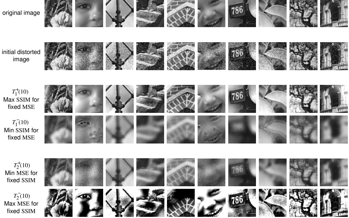
Figure 7. Synthesized images at initial distortion level l = 10 for performance comparisons of MSE and SSIM with variance-weighted pooling.
