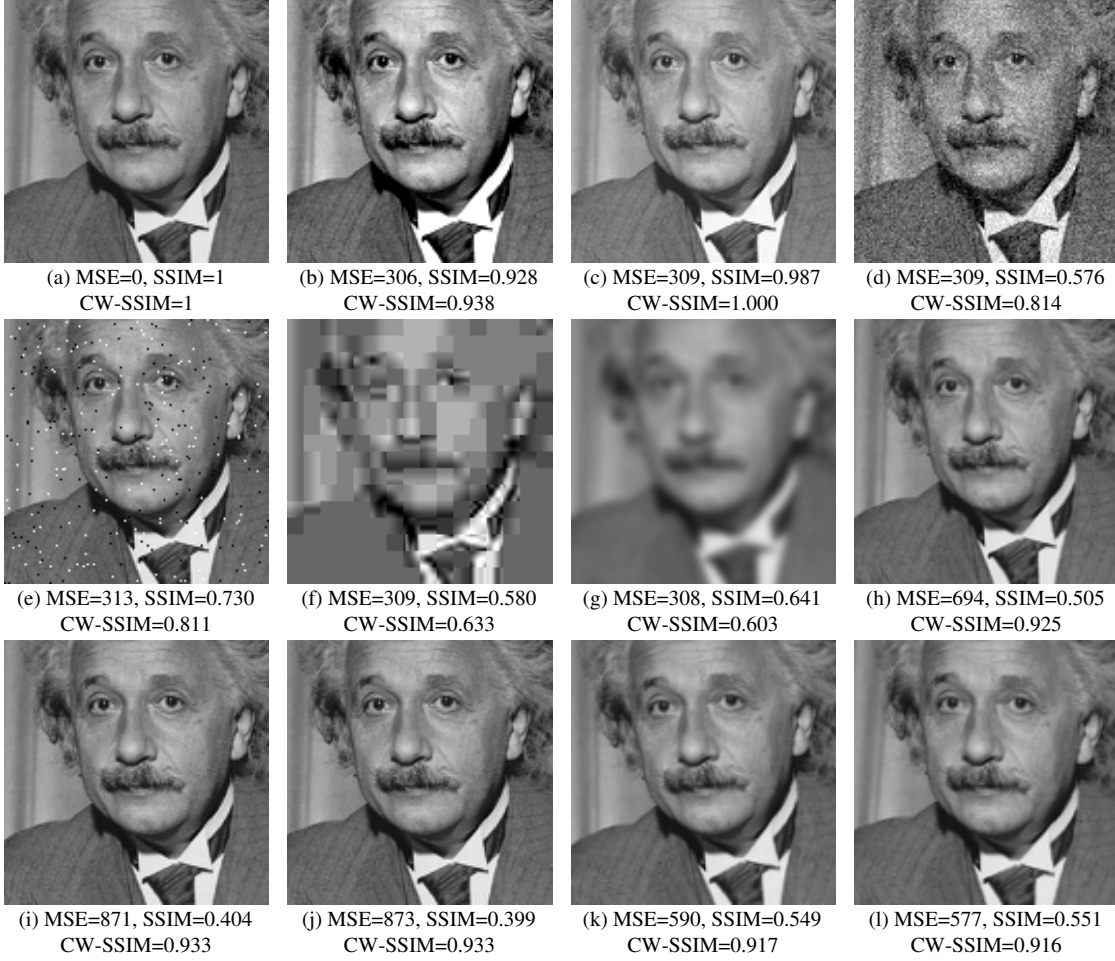
Fig. 1. Comparison of image similarity measures for images with different types of distortions. (a) reference image (8bits/pixel, assumed to have perfect quality); (b) contrast stretch; (c) mean luminance shift; (d) Gaussian noise contamination; (e) impulsive noise contamination; (f) JPEG compression; (g) blurring; (h) spatial scaling (zooming out); (i) spatial translation (to the right); (j) spatial translation (to the left); (k) rotation (counterclockwise); (l) rotation (clockwise). Images are cropped from 256 \times 256 to 128 \times 128 for visibility. Note that Images (b)-(g) have almost the same MSE values but drastically different visual quality, which is better predicted by SSIM and CW-SSIM. Also note that MSE and SSIM are both sensitive to translation, scaling and rotation (Images (h)-(l)), and CW-SSIM is robust to these distortions.
