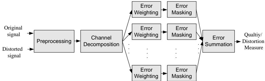
Fig. 1. Error sensitivity-based image/video quality measurement system.
