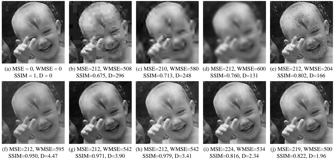
Fig. 2. Comparison of image distortion measures. (a) original image; (b) JPEG compression; (c) JPEG2000 compression; (d) blurring; (e) salt-pepper noise; (f) contrast reduction; (g) gamma distortion ( \gamma > 1 ); (h) gamma distortion ( \gamma < 1 ); (i) horizontal shift; (j) vertical shift.
