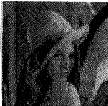
Fig. 7. The image after smooth region approximated by dc and linear approximation and edge blocks covered with their block mean
