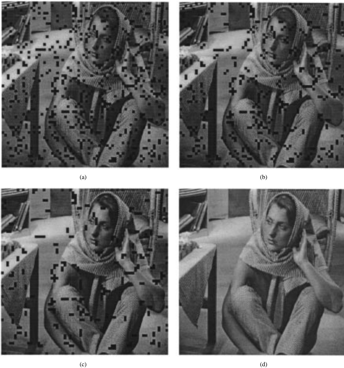
Fig. 4. (a) Damaged Barb image with contiguous block losses and with block loss rate of 15%, PSNR = 14.74 dB. (b) After Step 1, PSNR = 16.00 dB. (c) After Step 2, PSNR = 17.47 dB. (d) Reconstructed image after Step 4, PSNR = 32.84 dB.
