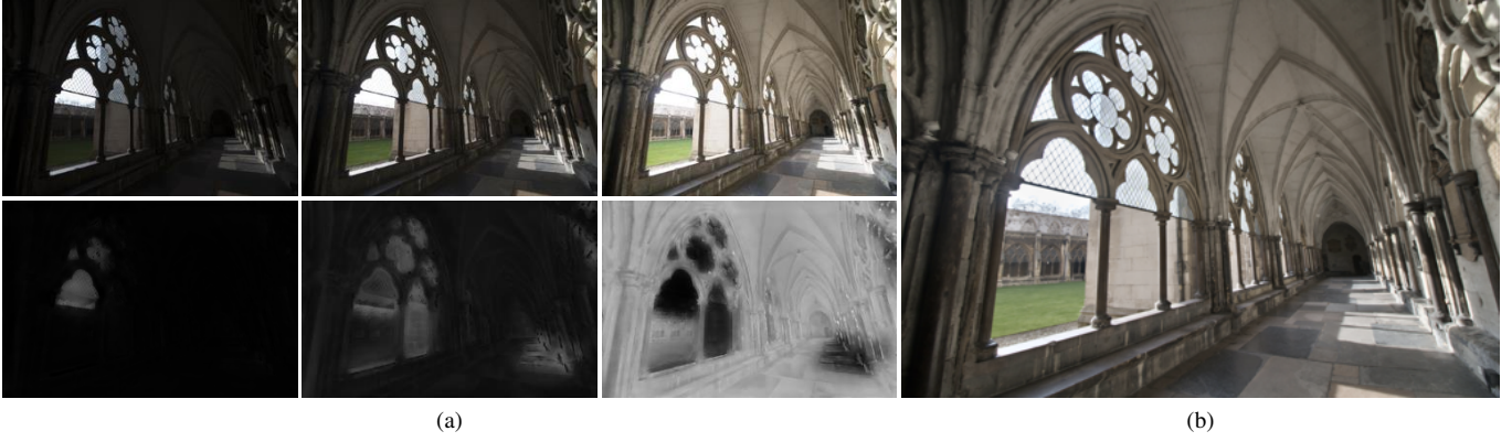
Fig. 2. Demonstration of the learned weight map \hat{\mathbf{W}}_k . A brighter pixel in \hat{\mathbf{W}}_k indicates that the corresponding pixel in \mathbf{X}_k contributes more to the fused image \mathbf{Y} . \hat{\mathbf{W}}_k shows a strong preference to high-contrast and well-exposed regions. (a) Source sequence ‘‘Corridor’’ along with the learned weight maps. (b) Fused image by MEF-Net. Sequence courtesy of Jianrui Cai.
