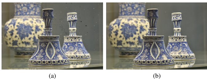
Fig. 10. Emergence of the dot artifacts with a small regularization parameter \lambda_a in the guided filter. (a) \lambda_a = 10^{-8} . (b) \lambda_a = 10^{-4} (default).
