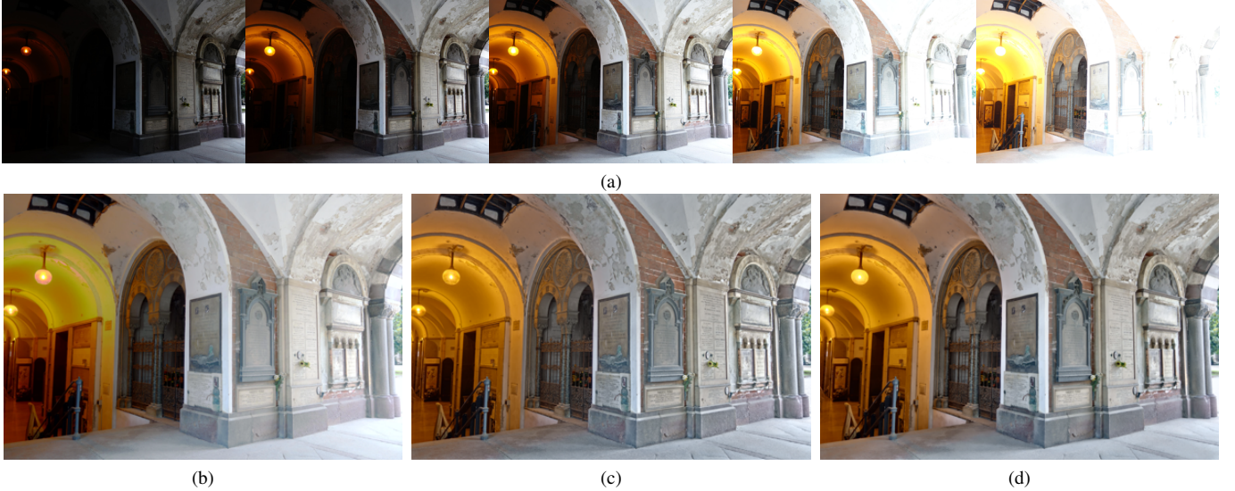
Fig. 6. MEF-Net in comparison with DeepFuse [6] and MEF-Opt [8]. (a) Source sequence “Archway” courtesy of Jianrui Cai. (b) DeepFuse. (c) MEF-Opt. (d) MEF-Net.
