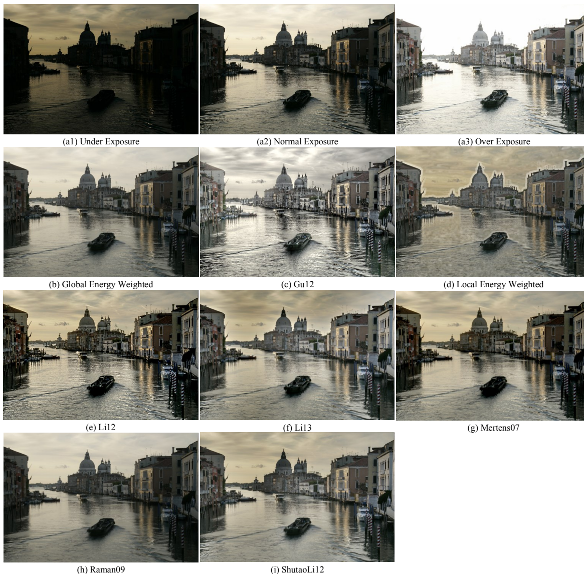
Fig. 2. An example of multi-exposure input images (a1, a2, a3) and fused images (b)-(i) created by different MEF algorithms.
