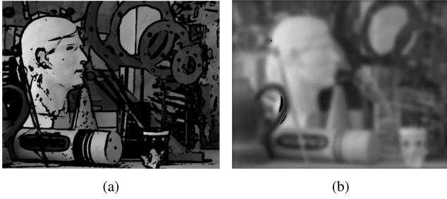
Fig. 6. Binocular Rivalry Example 1: The left-view is original and the right-view is blurred. The structural consistency between two-views is affected. The left-view may dominate the right-view at any time instance. (a) Left-view: Reference. (b) Right-view: Blur.
