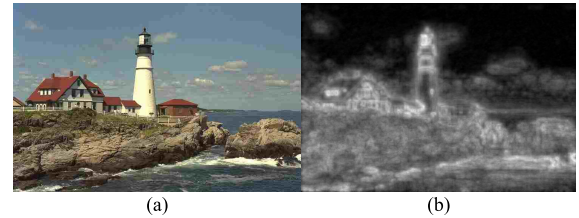
Fig. 10. Illustration of a JPEG compressed image at a bit rate of 0.4 b/pixel, and its corresponding natural scene saliency as the output of a saliency model (i.e., Torralba). (a) JPEG compressed image (b) Saliency map (i.e., Torralba) based on the original image of (a).
