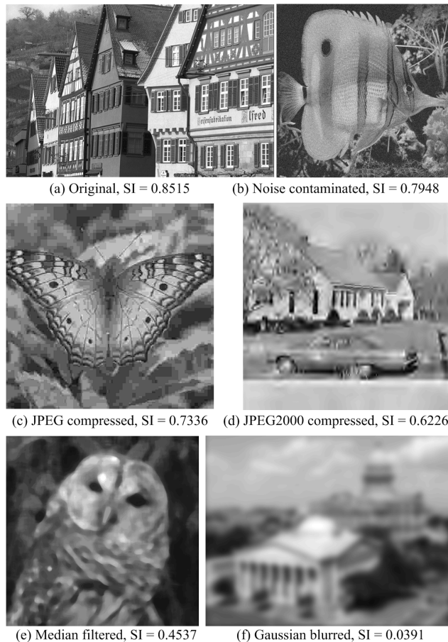
Fig. 4. Proposed sharpness index (SI) applied to (a) original distortion-free image; (b) white Gaussian noise contaminated image; (c) JPEG compressed image; (d) JPEG2000 compressed image; (e) Median filtered image; (f) Gaussian blurred image.
