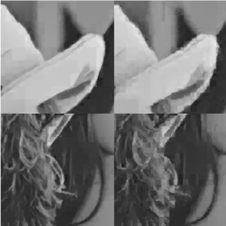
Fig. 7. Enlarged areas of 'Lena' image. Left: decoded image areas by the hybrid system; Right: quadtree decoded image areas.
