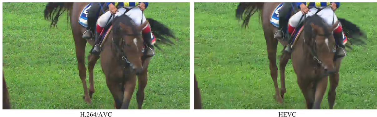
Fig. 4. An example of visual comparison between H.264-JM18.3 and HEVC-HM5.0 coded videos. Left: H.264 frame, PSNR = 28.36dB, SSIM = 0.8012, MS-SSIM = 0.8601. Right: HEVC frame, PSNR = 27.64dB, SSIM = 0.7437, MS-SSIM = 0.8259. When comparing individual frames, H.264 frame appears to have clearly better visual quality, but when the video is played at normal speed, the H.264 video receives a significantly lower quality score likely due to strong temporal artifacts.
